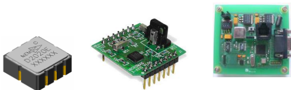
Fig. 4: Some of the sensors of the environment: accelerometer, magnetic sensor, high sensibility compass.
