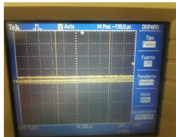
Fig.5.8 Faulty Optocoupler's Low side voltage output
