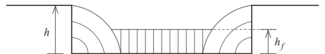
FIG. 6. Bent filled state approximated by two circular domains, of radius h , of nematic bent around the bottom corners connected by a flat layer of uniform homeotropic nematic, of height h_f .
