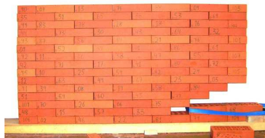
Figure 8. The wall after collapse.
