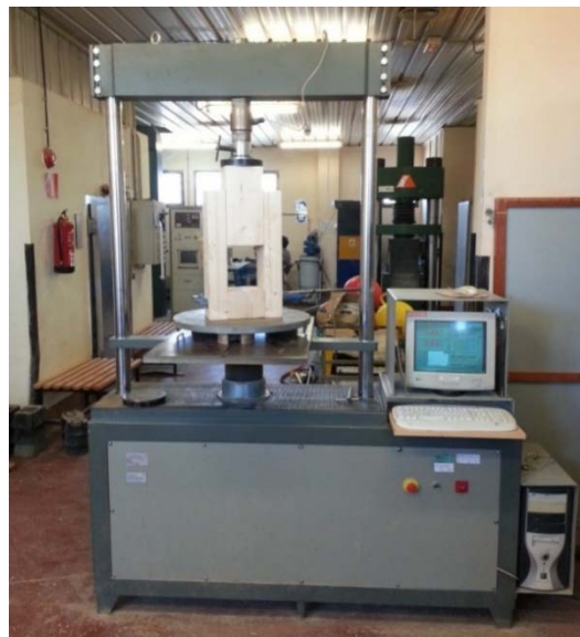
Figure 4. Composition of the sample in the testing machine.
