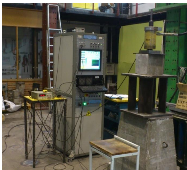
Figure 1. General view of the bond test arrangement
