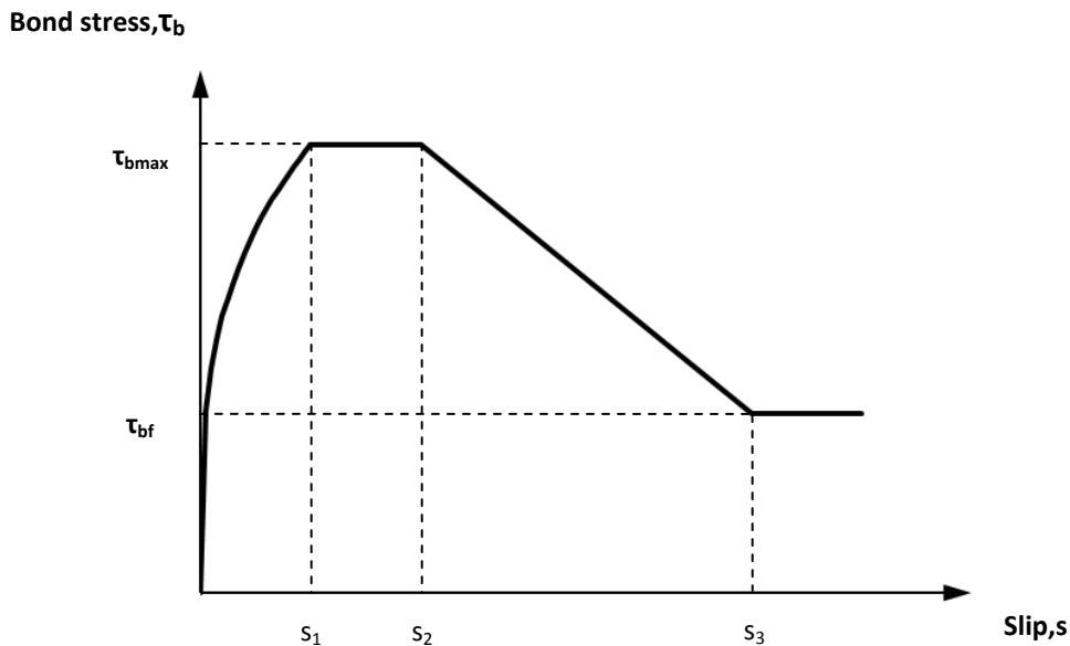
Figure 10. Bond-slip model proposed by Eligehausen et al.[19] and prescribed by the Model Code 2010 [20].
