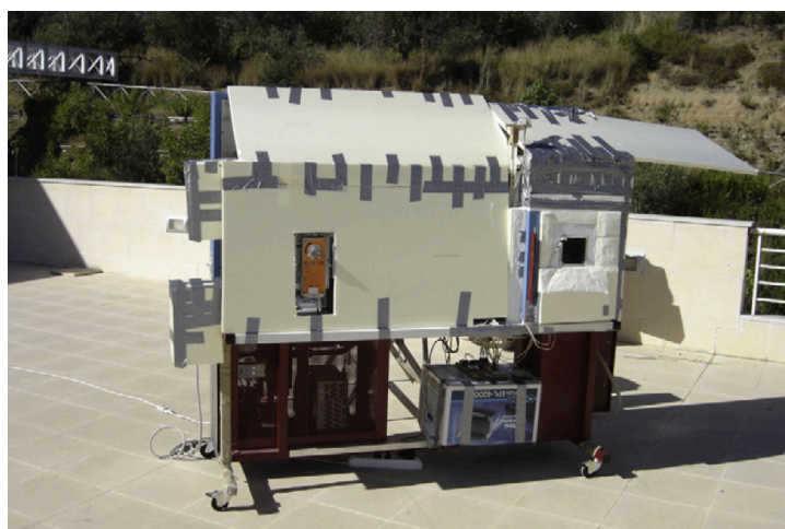
Fig.16. Células de ensayo. Fuente: A. Piccolo. "Thermal performance of an electrochromic smart window tested in an environmental test cell". Energy and Buildings . 2010.
