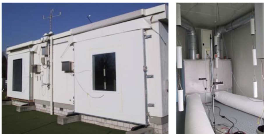
Figs. 9 y 10. Células de ensayo. Fuente: H. Manz, P. Loutzenhiser, T. Frank, P.A. Strachan, R. Bundi, G. Maxwell. "Series of experiments for empirical validation of solar gain modeling in building energy simulation codes—Experimental setup, test cell characterization, specifications and uncertainty analysis". Building and Environment . 2006.
