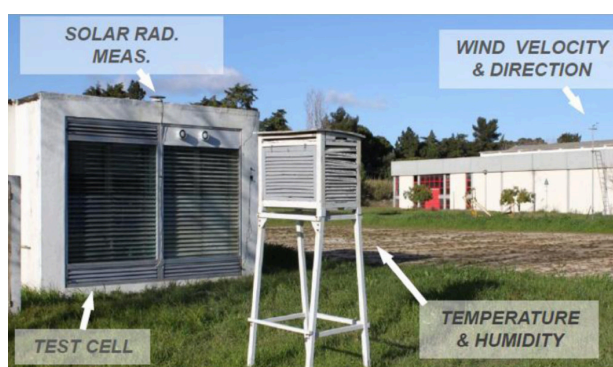
Fig.20. Células de ensayo. Fuente: Nuno M. Mateus, Armando Pinto, Guilherme Carrilho da Graca. "Validation of EnergyPlus thermal simulation of a double skin naturally and mechanically ventilated test cell". Energy and Buildings . 2014.
