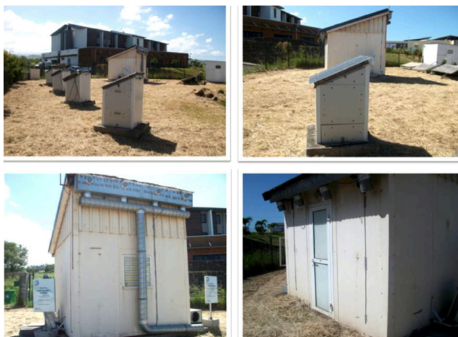
Fig.19. Células de ensayo. Fuente: André Bontemps, Maha Ahmad, Kevin Johannès, Hébert Sallée. "Experimental and modelling study of twin cells with latent heat storage walls". Energy and Buildings . 2011.
