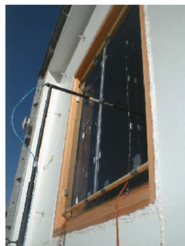
Fig.14. Células de ensayo. Fuente: V.Leal, E.Maldonado. "The role of the PASLINK test cell in the modelling and integrated simulation of an innovative window". Building and Environment , 2008.
