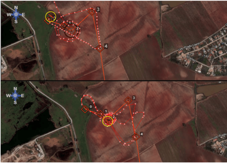
Figure 6.13 2D trajectory obtained when following the thermal flight plan proposed in Scenario 2. Up: Simulated; Down: Real.
