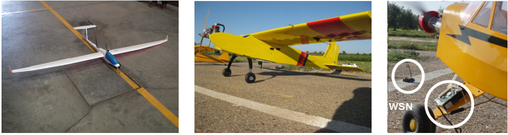
Figure 1.6 From left to right: fixed-wing gliding UAV used in experiments during the thesis; Megastar fixed-wing UAV; Piper fixed-wing UAV. Also, the on-board and deployed WSNs are detailed.
