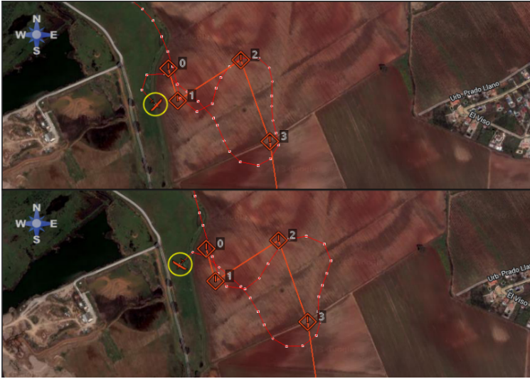
Figure 6.11 2D representation of the route obtained when executing the Scenario 1. Up: Simulated; Down: Real.
