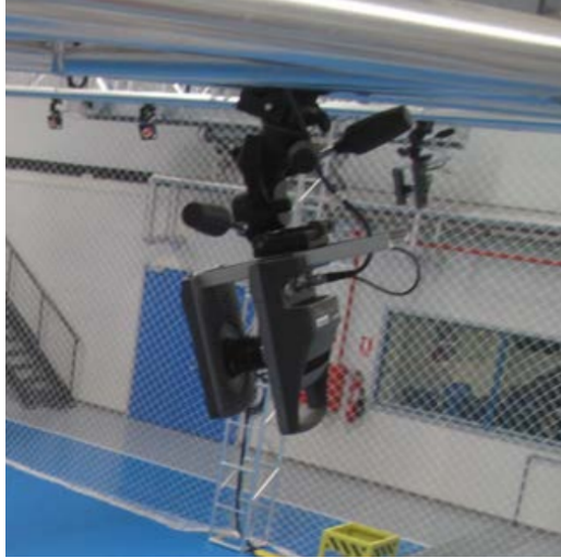
Figure A.2 Detailed of the IR cameras used by the VICON localization system.
