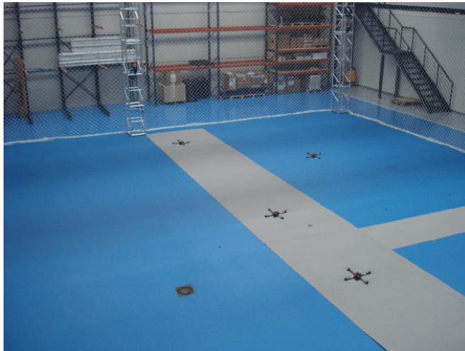
Figure A.1 Multi-UAV testbed located at the CATEC facilities when performing a Collision Avoidance experiment with 4 UAVs.
