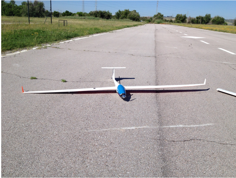
Figure 6.1 Gliding fixed-wing UAV used in the experiments.
