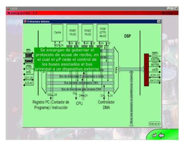
Fig. 6. TMS320C3X internal architecture description.
