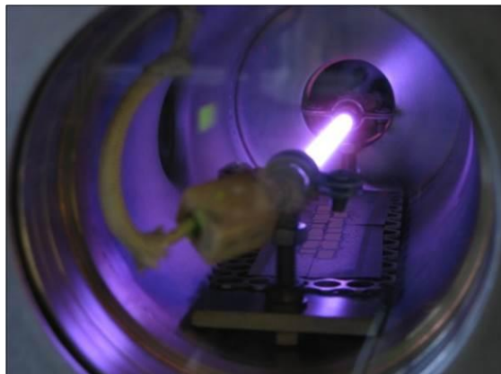
Figure 12. DC sputtering of Ag at the Nanotechnology on Surfaces group, ICMS.
