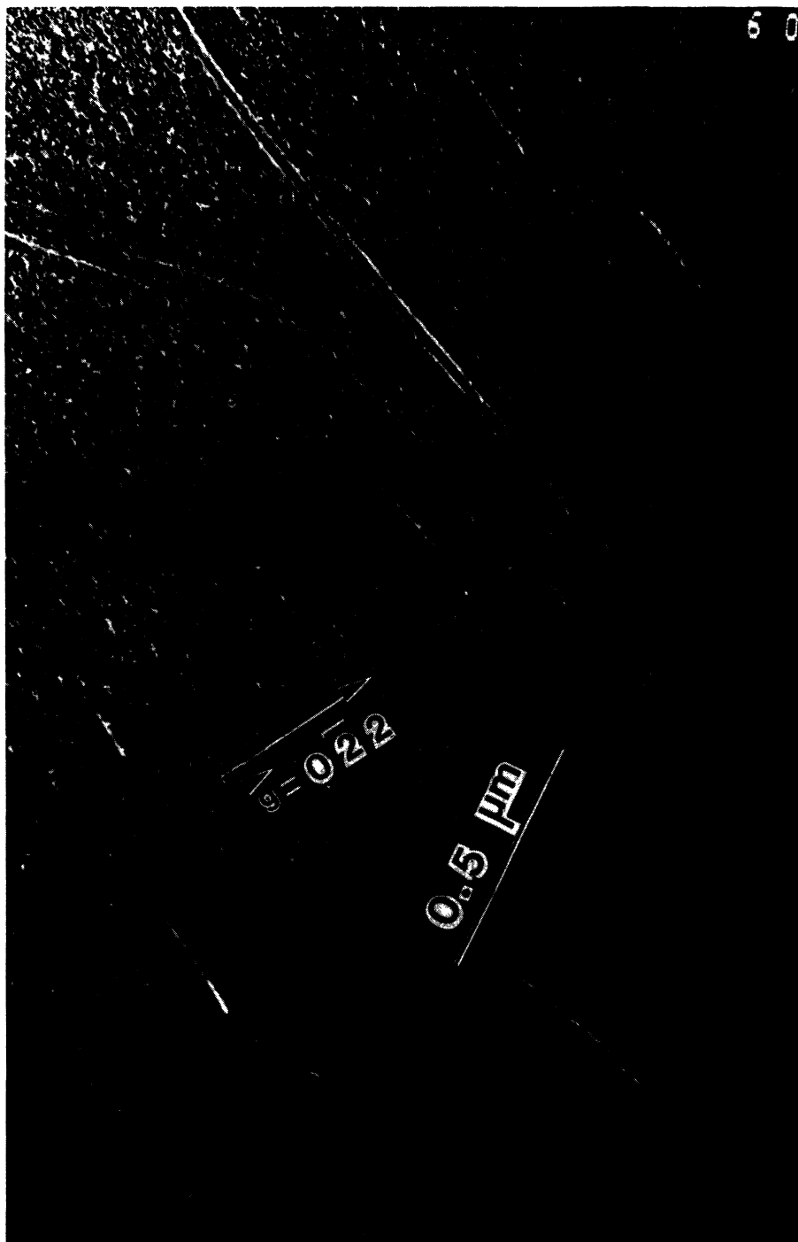
Fig. 5. — Weak beam dark field observation of an area next to the one of figure 4 with dipoles and multipoles. No dissociation for g = \pm 220 .
