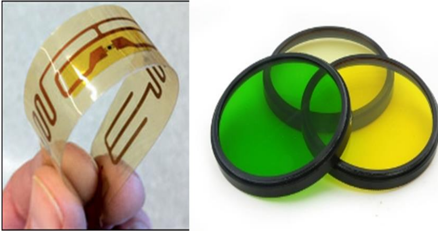
Figure 1.1- Some examples of thin film applications in microelectronics and integrated optics: (left) flexible electronic integrated circuit (right) optical filters.
