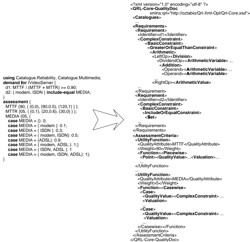
Figure 4. An example of a QRL-based demand written in XML.
