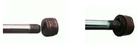
Figure 1: Pieces before and after the weld.
