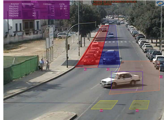
FIGURE 4: Detection areas in an installed prototype: details of the directional regions behavior (R3, R4, and R5) and queue detection areas (R1 and R2).
