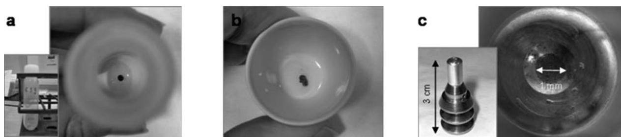
Fig. 2 Pictures showing the steps involved in the AMS cathode preparation process: (a) dry iron residue obtained after the evaporation of the purified plutonium solution with 1 mg of iron; (b) iron oxide obtained after baking at 800 °C the former residue; (c) images of the cathode where the final iron oxide plus aluminium mixture is pressed.
