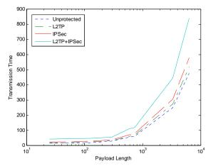
Figure 11 AH and ESP combined mode of transmission time simulation of Figure
