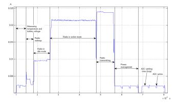
Figure 1. MSP430 working load in different operational modes, starting with the sensor measurement, the radio initialisation, radio listen mode (most power consuming), the transmission and the power management mode for preparing the deep sleep mode [2].
