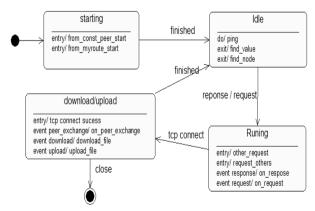
Figure 1. the node process transition
