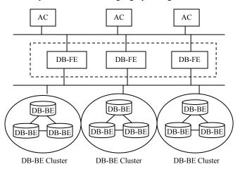
Figure 1. The middleware-based replication architecture for high availability database applications
