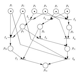
Figure 4. A Petri net model of a WSN.
