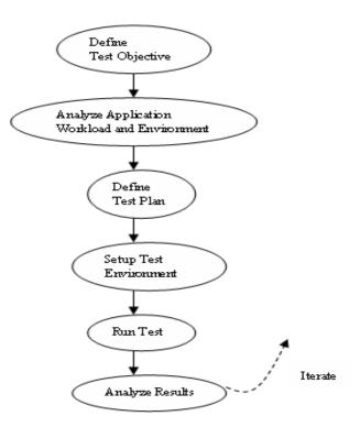
Figure 17: Major Phases of the Performance Testing Process.
