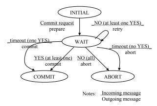
Figure 7. Coordinator 's state transition diagram
