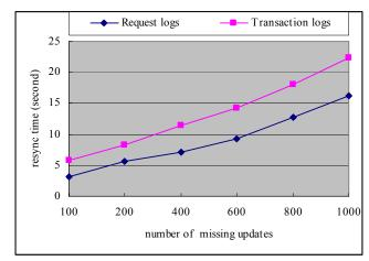
Figure 13. Comparison of resynchronization time
