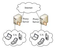
Figure 1. Simplified configuration of a SIP network.
