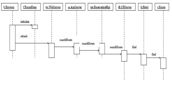
Figure 8. Sequence diagram of the Reservation System - Room search scenario.
