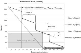
Figure 11. Single hop communication example. Comparison between a conventional ZigBee communication and buffered communication scenarios both with and without WuRx capabilities. The different operational modes for the local data measuring and the data transmission are marked. Our goal is to maximise the system availability and to minimise the power consumption during the autonomous measuring *mode A*, represented by the term  $\frac{\Delta E}{\Delta t}$ .
