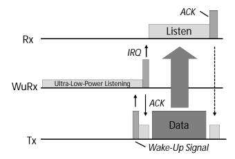
Figure 3. Wake-up receiver communication. The main network interface is waiting in a standby mode and will be activated by the WuRx on demand. The WuRx is designed as an ultra-low-power component, which only has to detect a predefined, coded wake-up signal from its environment.
