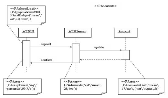
Figure 4. Performance annotation for a deposit scenario at a cash machine - Sequence diagram.
