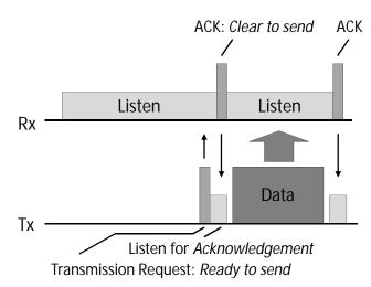
Figure 2. Conventional communication process between transmitter (Tx) and receiver (Rx). The receiver has to sense the medium. Dependent on the transmission parameters and the characteristics/duty cycle of the used radio standard, this listening mode consumes a lot of energy.
