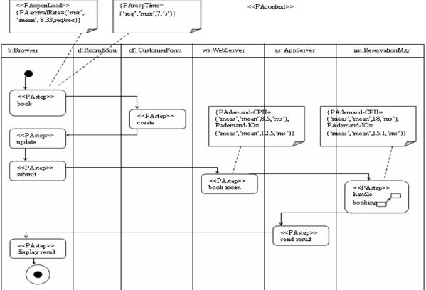
Figure 14. Annotated activity diagram for the Reservation System- Reservation confirmation scenario.
