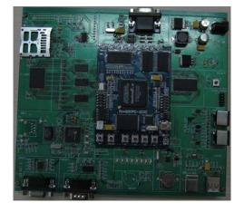
Figure 10. Development board based on new high secure architecture of network computer
