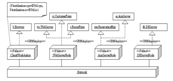
Figure 16: Annotated deployment diagram for the Reservation System.
