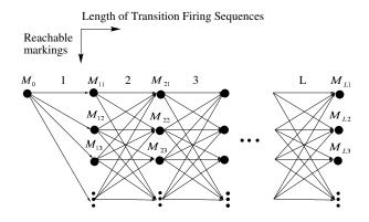
Figure 2. Trellis diagram of the evolution of reachable markings.
