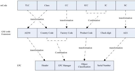
Figure2. The process of transforming mCode into EPC
