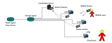
Figure 6. Set up for the live demo. All terminals (LT1, LT2, CN), the Foreign Agent and the Localization Server lie on the same local network; the Home Agent is co-located with the Proxy and is one hop away the Foreign Agent.
