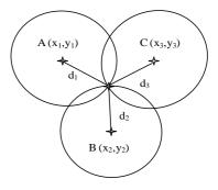
Figure1. The model of Nodes' localization
