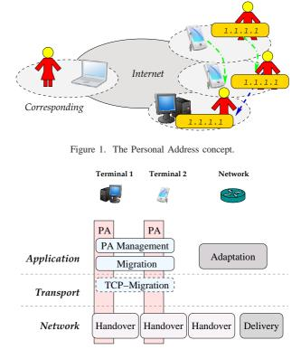
Figure 2. The architecture of the user-centric mobility framework based on the Personal Address.
