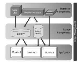
Figure 7. The power management is responsible for an efficient usage of the available energy resources and the harvesting components. In combination with an intelligent application design and modern WuRx technology, the system availability increases significantly.
