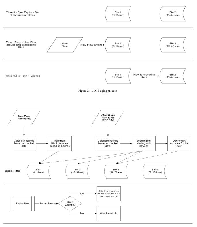
Figure 3. Flow chart of the life of a flow in BDFT
