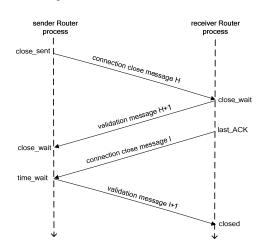
Figure 9. The process of closing connection
