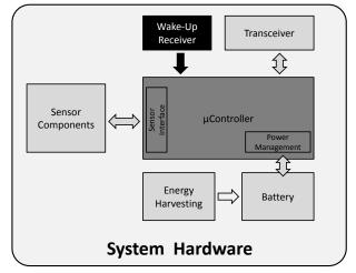
Figure 5. Typical system hardware architecture of an embedded system with a wake-up receiver unit.
