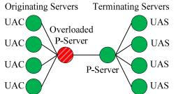
Fig. 2. SIP network topology with an overloaded P-server (which is marked in diagonal lines) and its multiple upstream originating servers.
