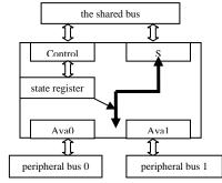
Figure 2. Structure of bus bridge
