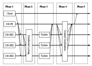
Figure 2. Synchronous update everywhere replication model
