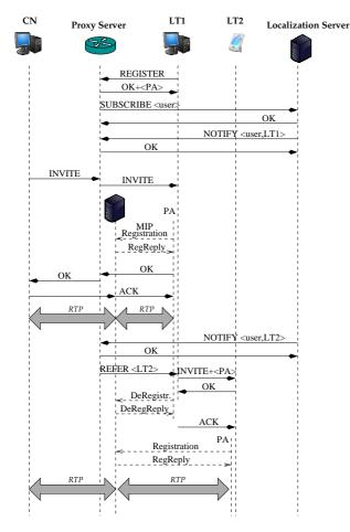
Figure 5. SIP signaling for session set-up and migration in the mobility framework.
