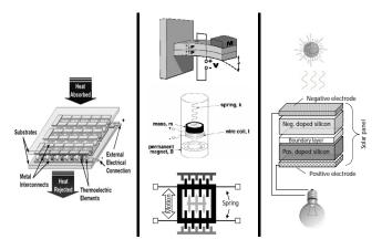
Figure 6. Typical energy harvesting technologies - Thermoelectric converter (left); Photovoltaic converter (right). Vibration-based converter elements (center) can be separated into: Piezoelectric harvesters (top); Electromagnetic harvesters (center); Electrostatic harvesters (bottom).
