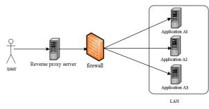
Figure 7: Reverse Proxy Structure
