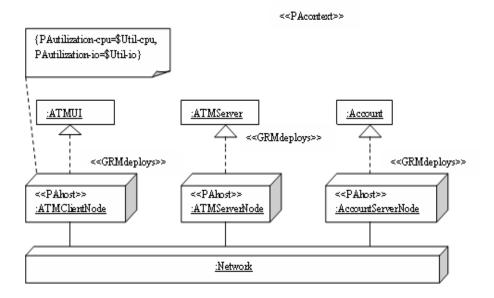
Figure 5. Performance annotation for a deposit scenario at a cash machine - Deployment diagram.
