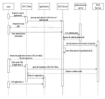
Figure 2: The whole process of Single Sign-on
