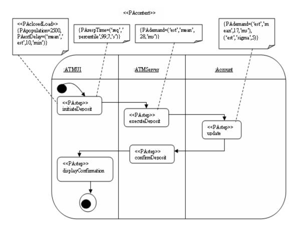
Figure 6. Performance annotation for a deposit scenario at a cash machine - Activity diagram.
