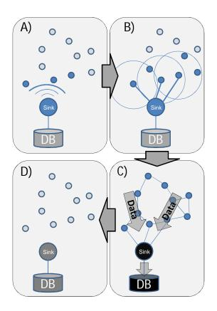
Figure 13. Application scenario - operational schedule with four steps. A) initial wake-up signal from the data sink in order to collect data from each sensor node. B) recursive wake-up signal from active nodes to explore the topology. C) Multi-hop data transmission of the measurement data over the established network topology. D) Communication finished, return to the autonomous mode without network infrastructure and waiting for new WuRx events.
