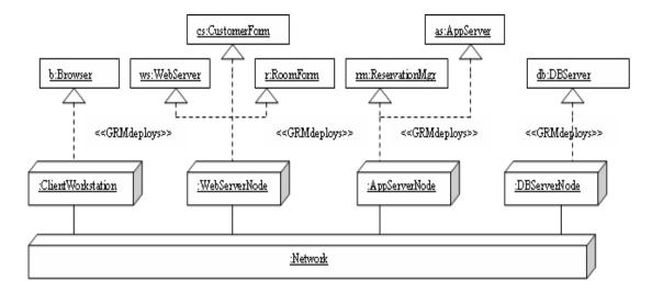
Figure 11. Deployment of the logical elements on the hardware infrastructure for the Reservation System.
