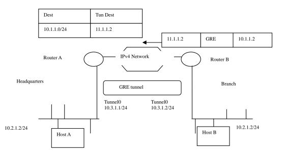
Figure 5 Dynamic Tunnel destination address
