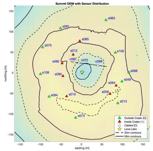
Figure 2.1 Digital elevation model (DEM) of Villarrica's summit showing locations of 20 sensors.
