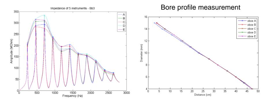
Differences in the impedance partially explained by discrepancies in the bore profiles.
