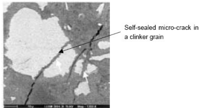
Fig. 2.8 Self-healing of UHPC micro-crack [Acker and Behloul, 2004]
