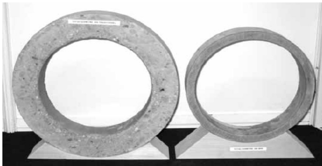
Fig. 2.23. Reduction in pipe wall thickness of UHPC (right) compared to an equivalent pipe with normal concrete (left) [Droll, 2004]
