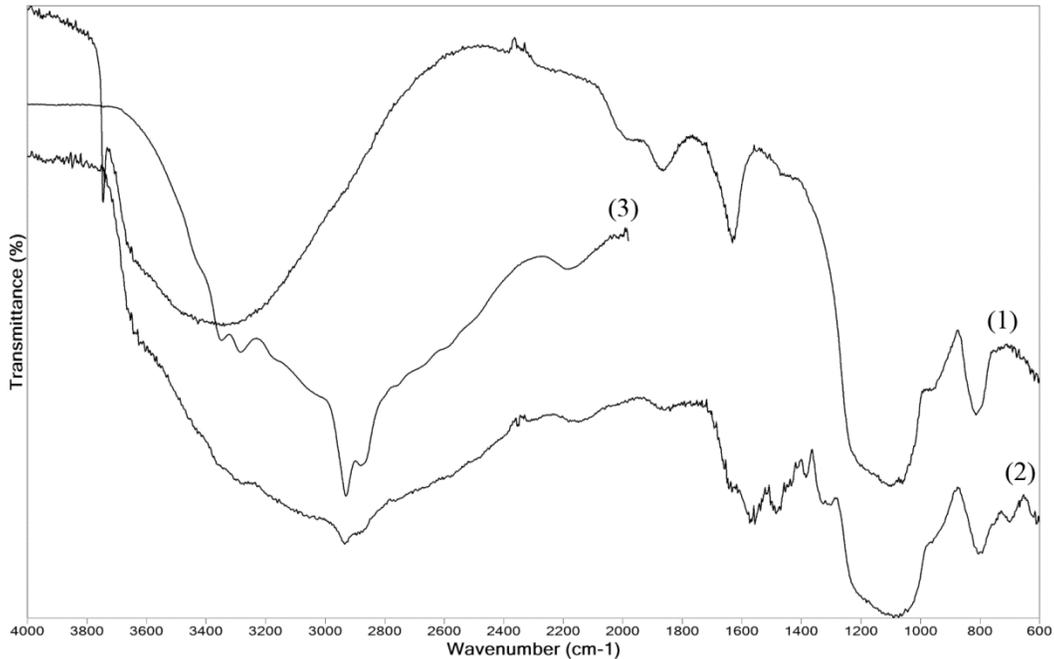
Figure 7-3 : FTIR spectra of raw silica fume (1), functionalized silica fume (2) and APTMS on glass substrate (3)
