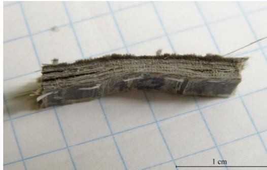
Figure 7-7 : Macroscopic mode of failure after ILSS test
