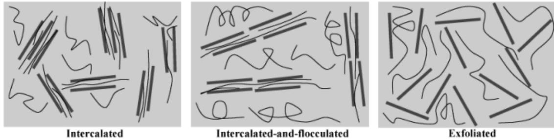
Figure 5-2 : Schematic illustration of the three main classes of polymer/organosilicate composites [137]
