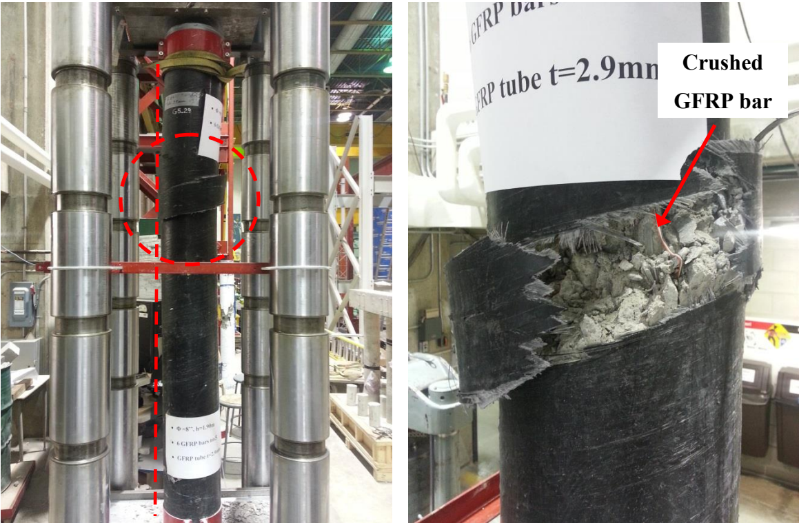
Figure 4.4: Failure mode of specimen A-G (3.4) -C
