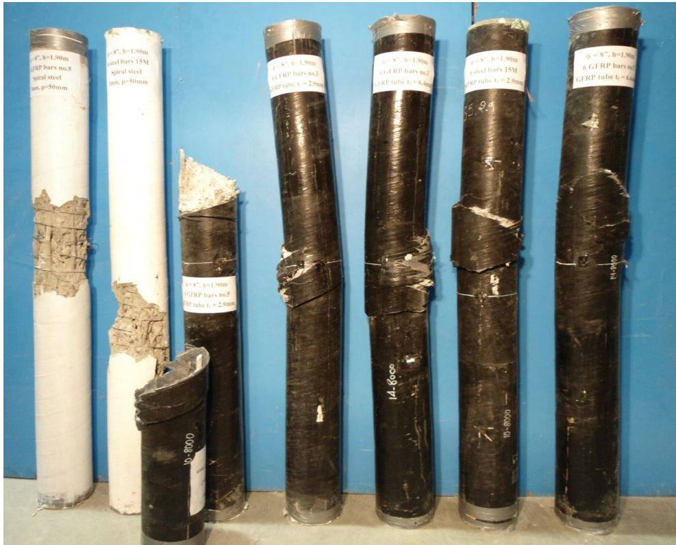
Figure 4.9: Overall failure modes of tested specimens
