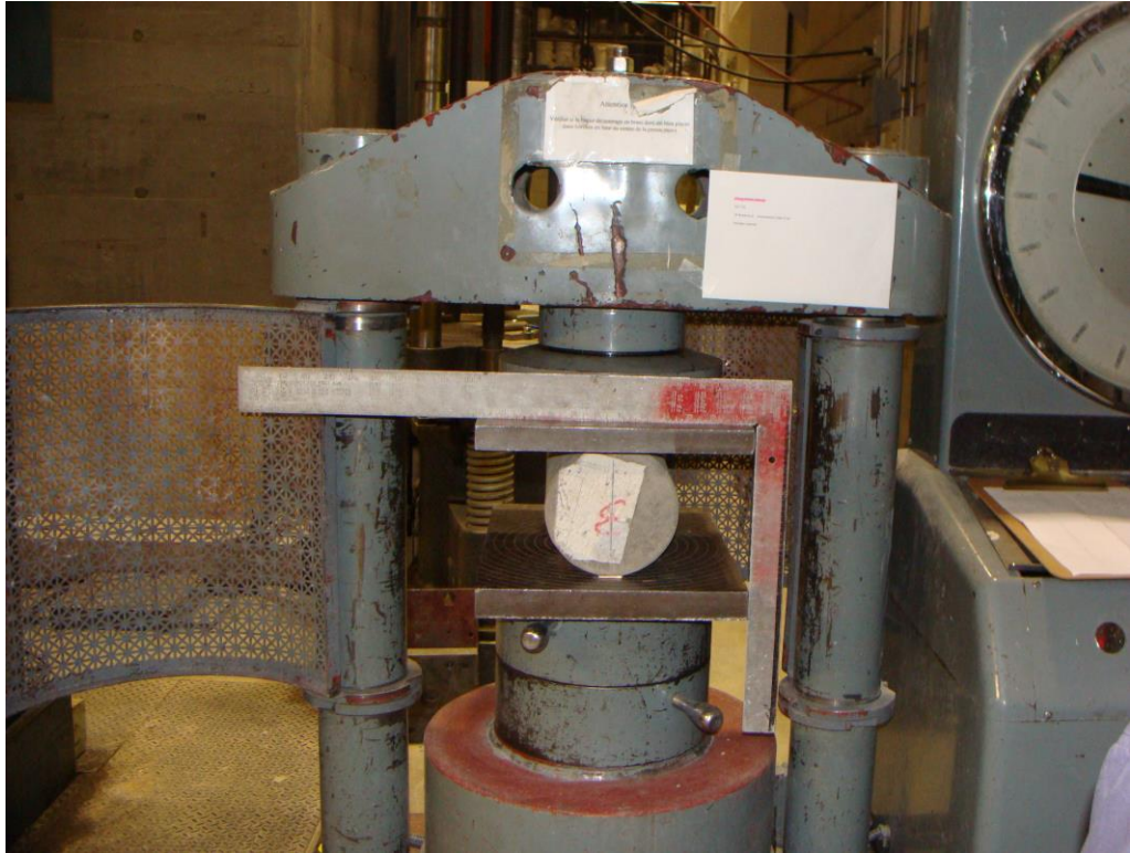
Figure 3.2: Splitting test of the standard concrete cylinders
