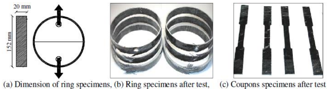
Figure 2.6: Specimens of FRP tubes for the split-disk test and coupon tensile test (Masmoudi and Mohamed 2011)
