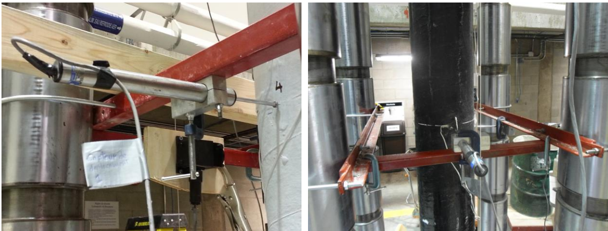
Figure 3.11: Horizontal LVDTs for measuring the lateral displacements
