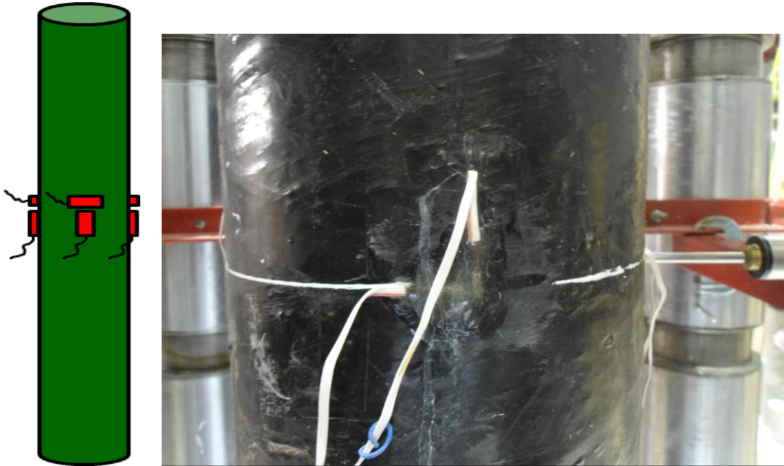
Figure 3.10: Vertical and horizontal strain gauges
