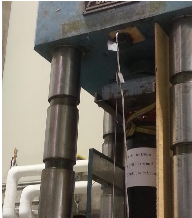
Figure 3.12: Vertical DTs for measuring the axial displacements
