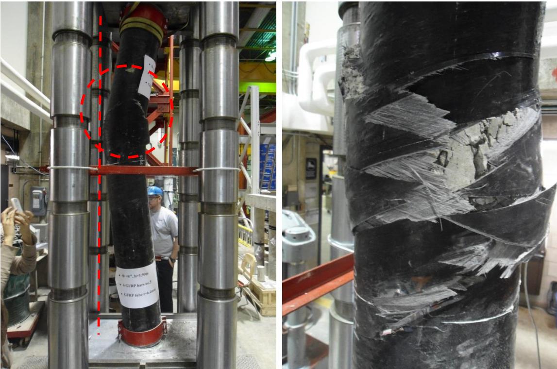
Figure 4.5: Failure mode of specimen B-G (3.4) -C
