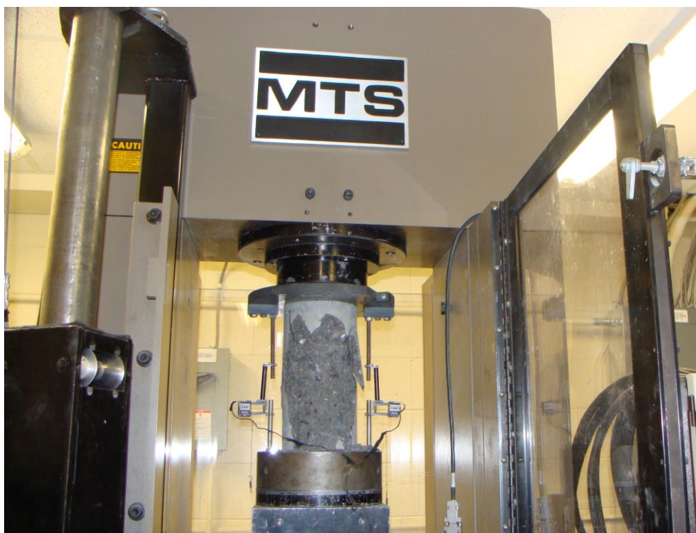
Figure 3.1: Compression test of the standard concrete cylinders
