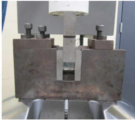
Figure 3–3: Typical test setup for transverse-shear tests
