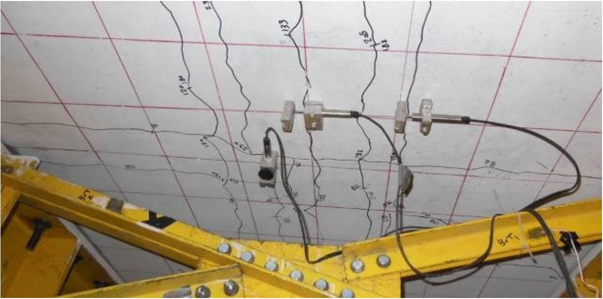
Figure 3–28: LVDTs to record the crack widths
