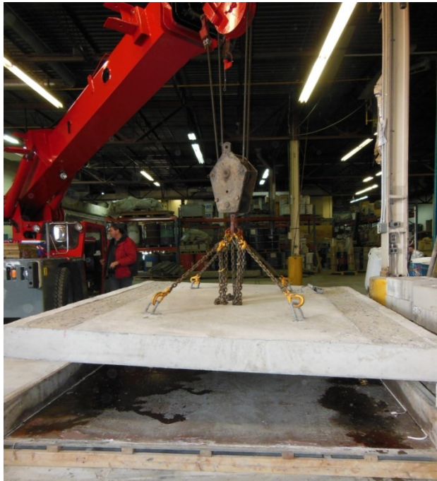
Figure 3–22: De-molding of the concrete deck slabs
