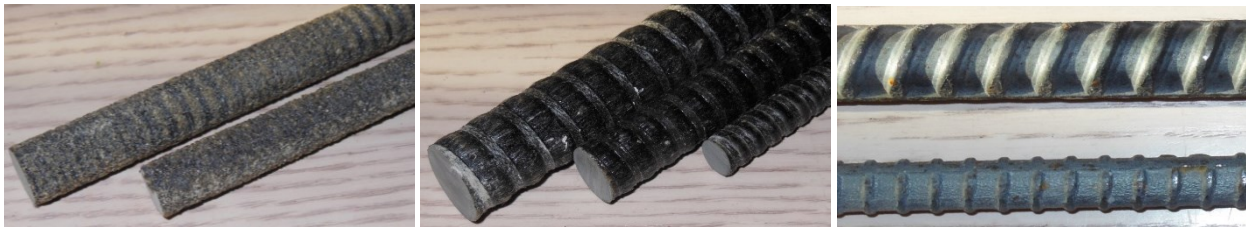
BFRP bars used in Chapter 6 BFRP bars used in Chapter 7 Steel bars used in Chapter 7
