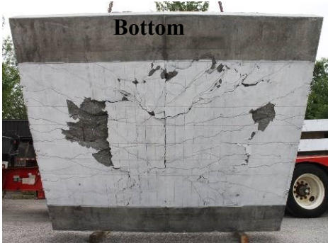
Figure 5-7: Cracks pattern at failure
