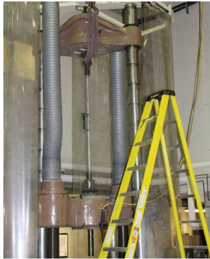
Figure 3–2: Typical test setup for tensile tests
