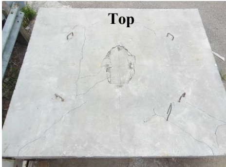
Figure 5-7: Cracks pattern at failure
