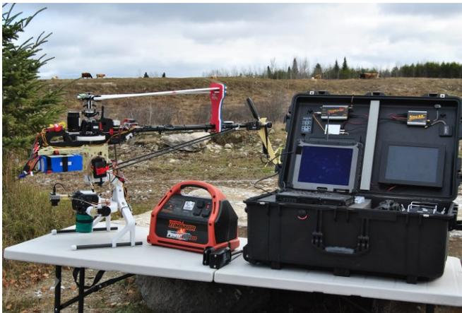
**Figure 31. Ground control station and unmanned aerial vehicle used in this study (Responder, ING Robotic Aviation)**
