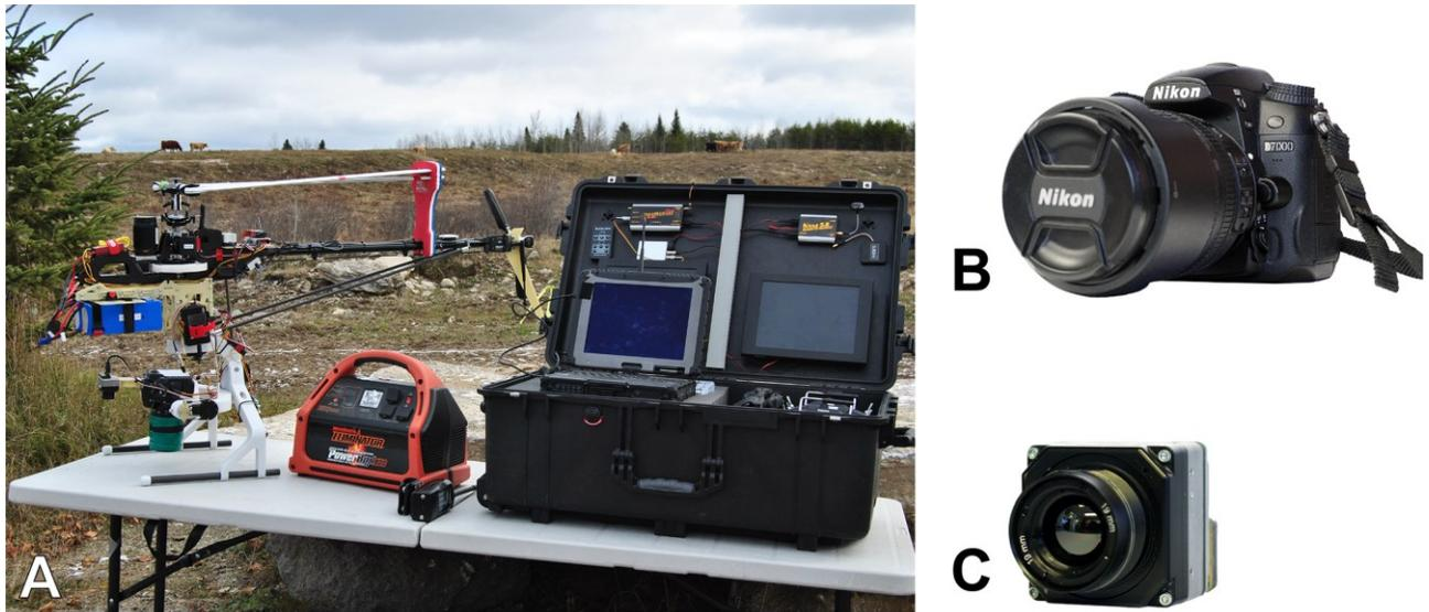
**Figure 24. Equipment used: A. Unmanned aerial vehicle and ground control station (ING Robotic Aviation, Sherbrooke, Canada); B. D7000 visible sensor (Nikon Inc., Tokyo, Japan); C. Tau640 thermal infrared sensor (FLIR Systems, Wilsonville, USA). Photo credits: CGQ and E. Gavelle**
