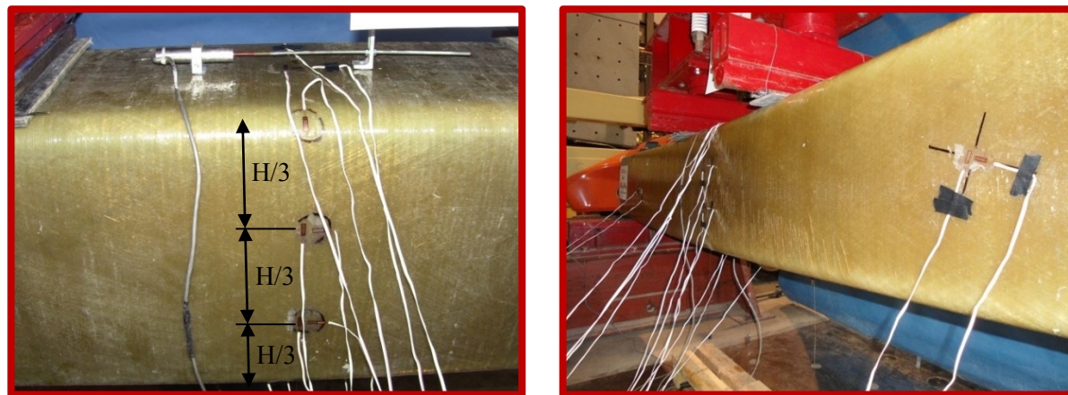
(a) Axial and hoop strain on outer tube
