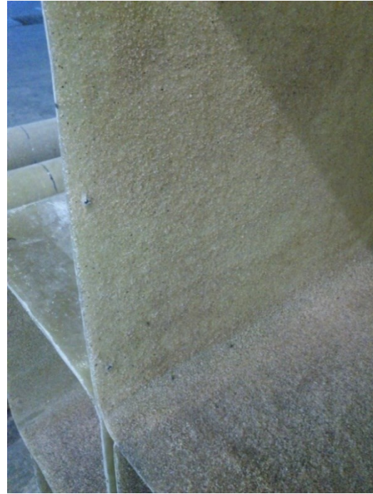
(b) Sand coating the inner surface of outer tubes
