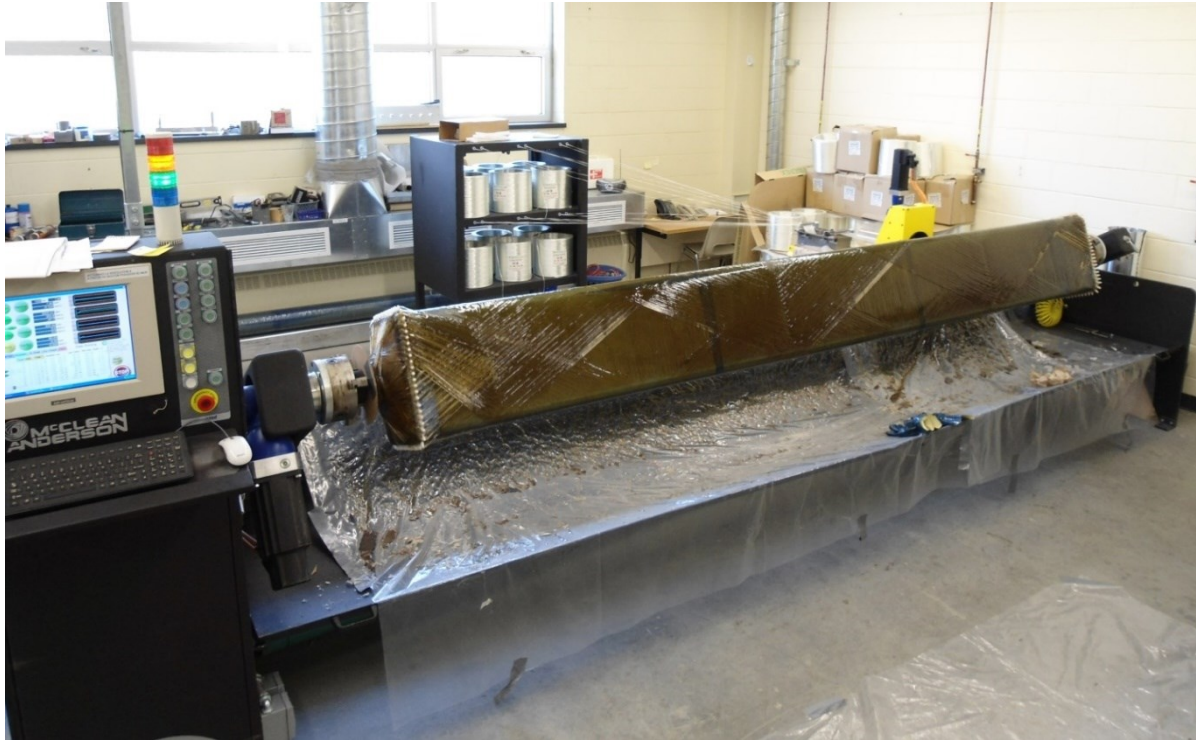
Figure 3.1 – Filament winding process (Civil Engineering department, Sherbrooke University)
