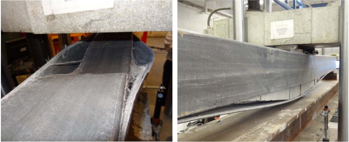
Figure 4.4 – Corner failure in pultruded FRP tubes (Belzer et al. 2013)
