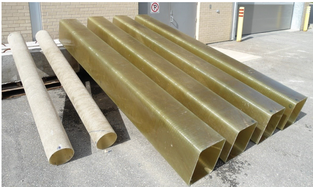
Figure 3.6 – Final Products of GFRP tubes
