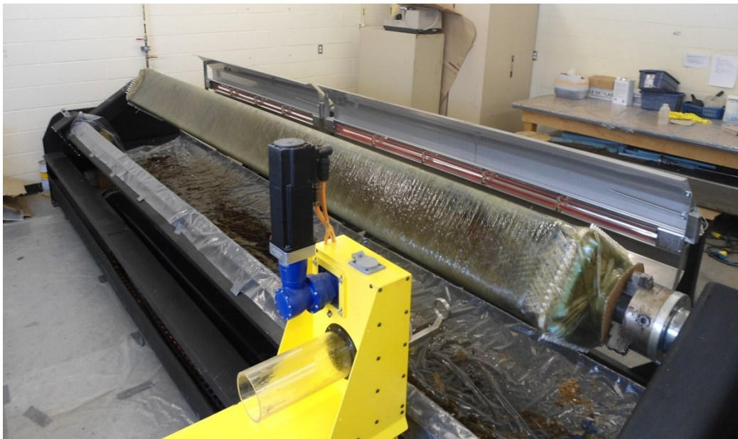
Figure 3.4 – Curing of FRP tubes by applying heat
