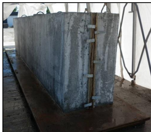
Figure 3.7 - Test specimen after the removal of forms
