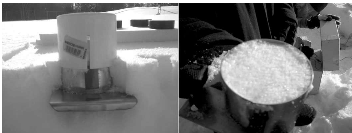
Fig. 2. The IRIS sampler before extraction of the snow sample within the snow cover (left) and after the sample extraction with the cut surface (right).
