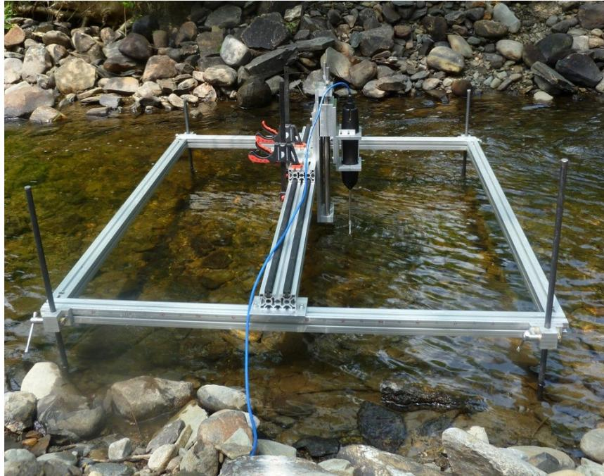
**Figure 4.3 - Field mounting frame for the ADV (flow direction from right to left)**
