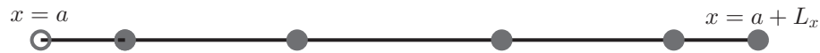
Figure 2.29 The unit cell of one dimensional element for numerical dispersion analysis, for a 6 nodes Legendre spectral element
