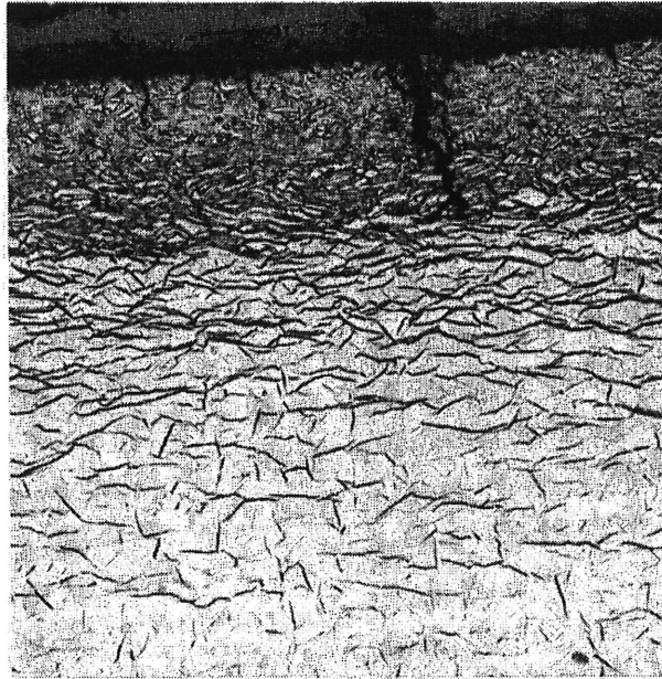
Figure 4. Photomicrograph of severely hydrided unalloyed titanium at the magnification of 200 \times (54).
