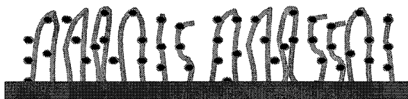
Figure 2.7: CMD chains having COOH groups (black dots) grafted on the surface with a carpet-pile like structure
