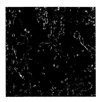
Figure 4.22: Texture Image of Selected Second-order Features for G2 Specimen: Mean Variance, Homogeneity
