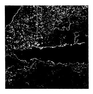
Figure 4.36: Texture Image of Selected Second-order Features for Spalling Image: Mean, Variance, Contrast
