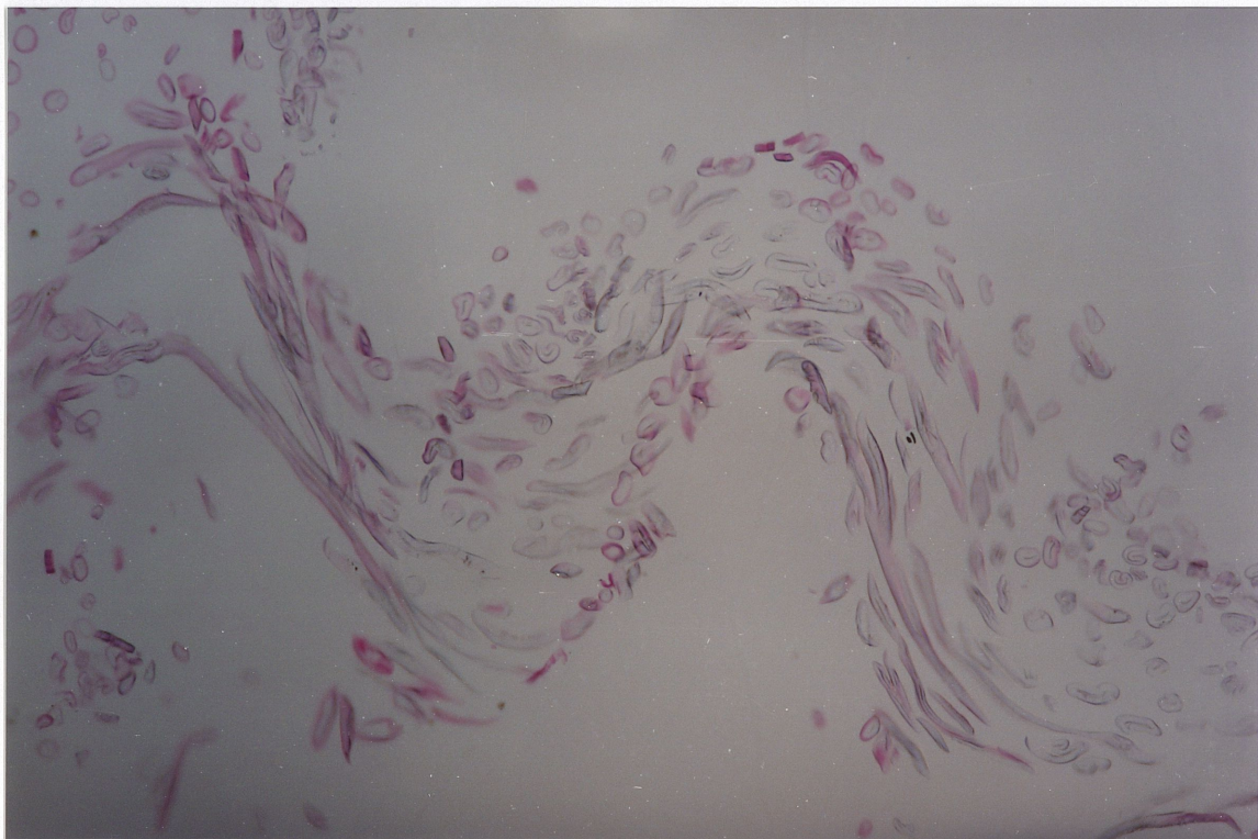
Figure 6.14 Cross section of dyed cotton fabric by optical microscope for Drimarene Red X-6BN in hot air fixation at 172°C
