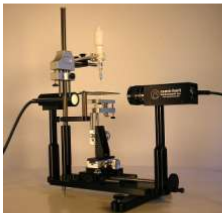
Figure A. 4 Schematic of ramé-hart contact angle goniometer used to measure CA
