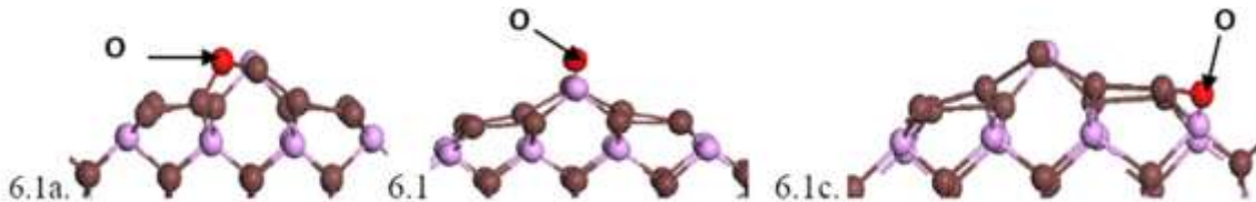
Figure 2. 17 View of oxygen adsorption on the InP (100). In, P, O, are indicated by brown, pink, and red spheres, respectively [K. Santosh, et al. 2013].
