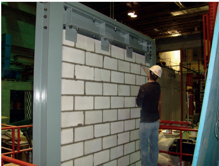
Figure A.4 Tirage de joints - Mur 1
