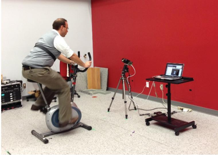
Figure 5.8 Experimental settings with the exercise bike, the thermal camera on the tripod and the GUI station.
