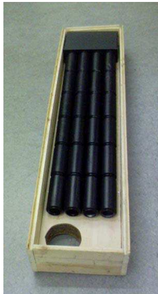
Figure 8.3. The structural view of the solar air heat collector (Photo by Edina Juhász)
