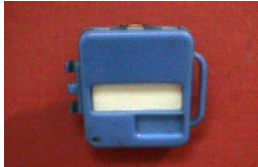
Figure 12.1. Film dosimeter holder (blue) and the film (white) in it.
