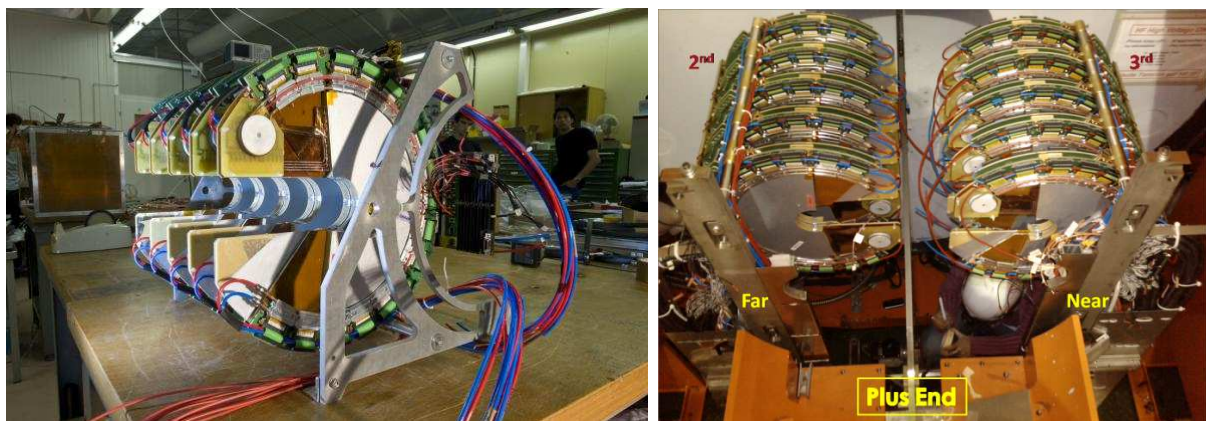
Figure 1.10: Half arm of the T2 detector (left) and the two halves of a single arm of the T2 detector before installation (right).
