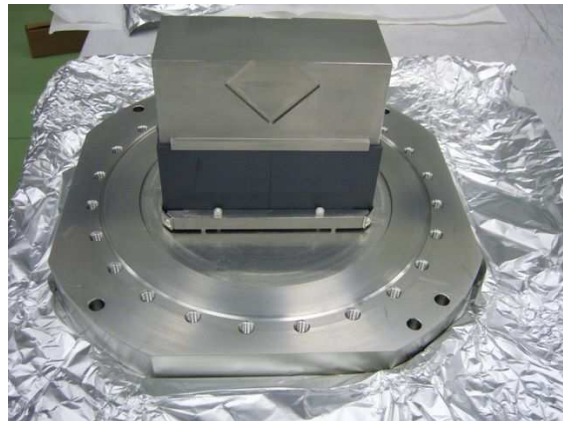
Figure 1.5: Roman Pot with the diamond shaped thin window and with the ferrite collar mounted around the housing on the beam vacuum side.
