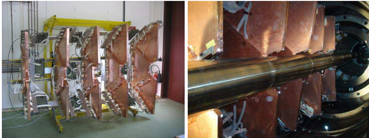
Figure 1.9: Half arm of the T1 forward telescope before (left) and after (right) installation inside the endcaps of the CMS detector.
