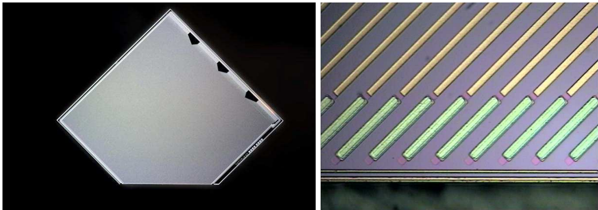
Figure 1.8: Planar Edgeless Detector with CTS (left). The magnification of a portion of the chip cut region (right) shows the details of the CTS.
