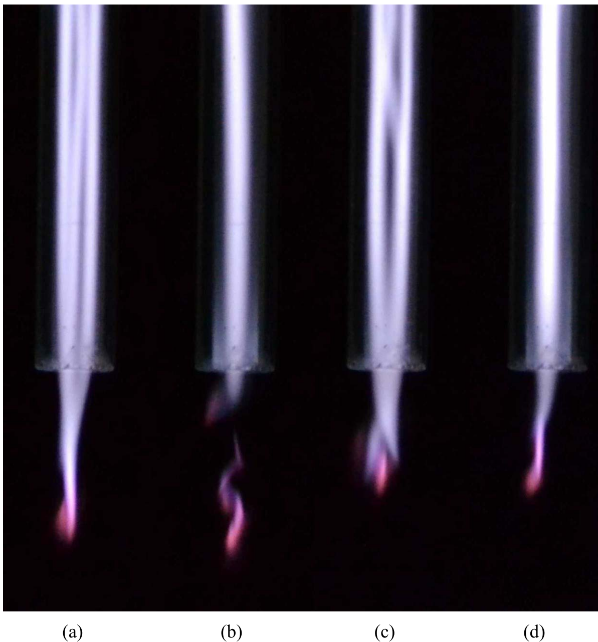
Fig. 1. Side view of the tip of the microwave plasma jet in argon with AM input power (265-Hz AM frequency, rectangular envelope-150 W in minimum, 350 W in maximum, and duty cycle 1:1). Exposure time 250 \mu\text{s} , ISO 3200. Sequence of the images was taken in different phases of the modulation envelope [(a) = 1 ms, (b) = 2 ms, (c) = 3 ms, and (d) = 4 ms]. At the falling edge of envelope (second image from the left), the plasma plume end separates from the bulk plasma.
