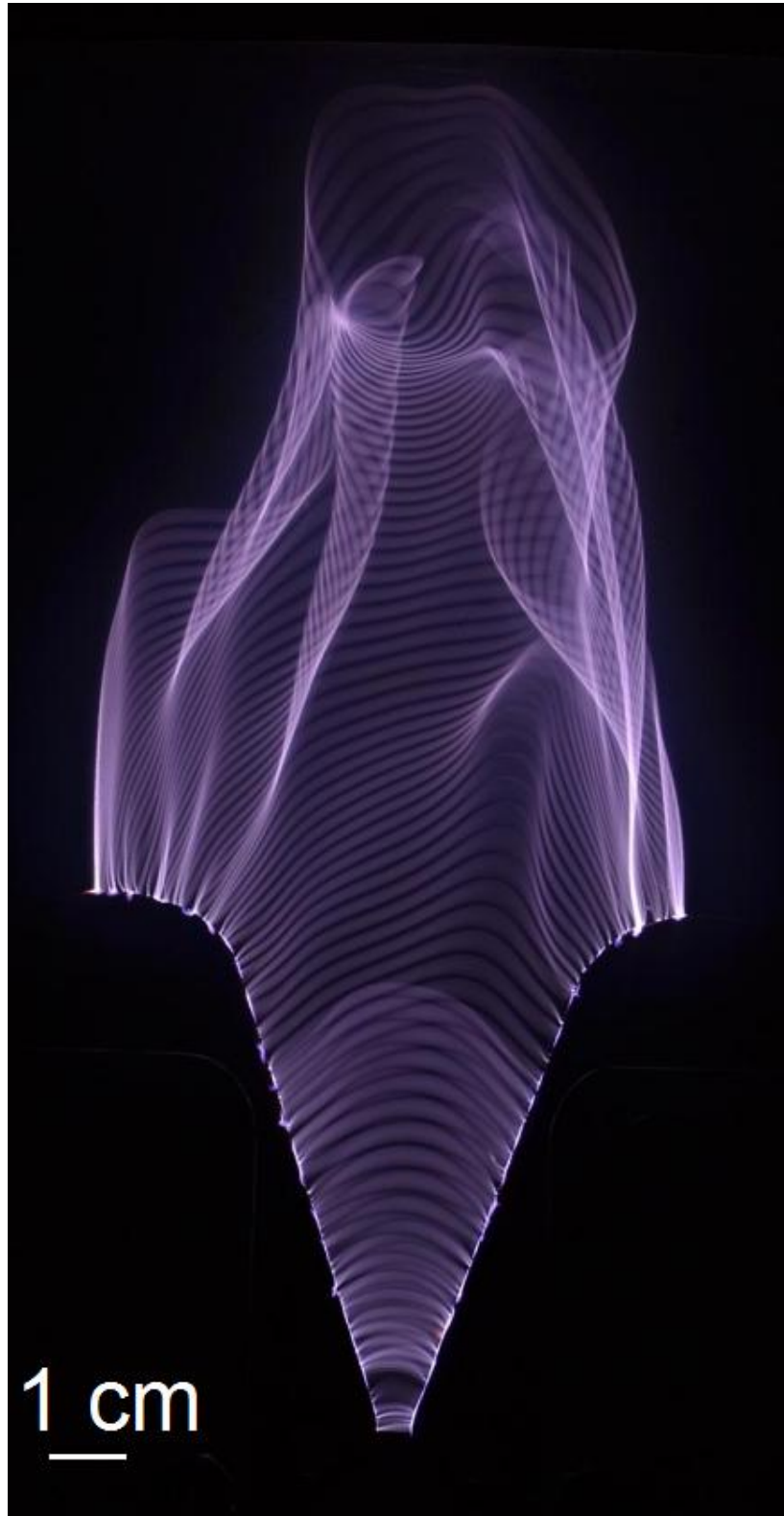
Fig.4: Long exposure (1 s) photograph of glide arc in argon (argon gas flow 0.4 slm; discharge voltage 4 kV; 1g).
