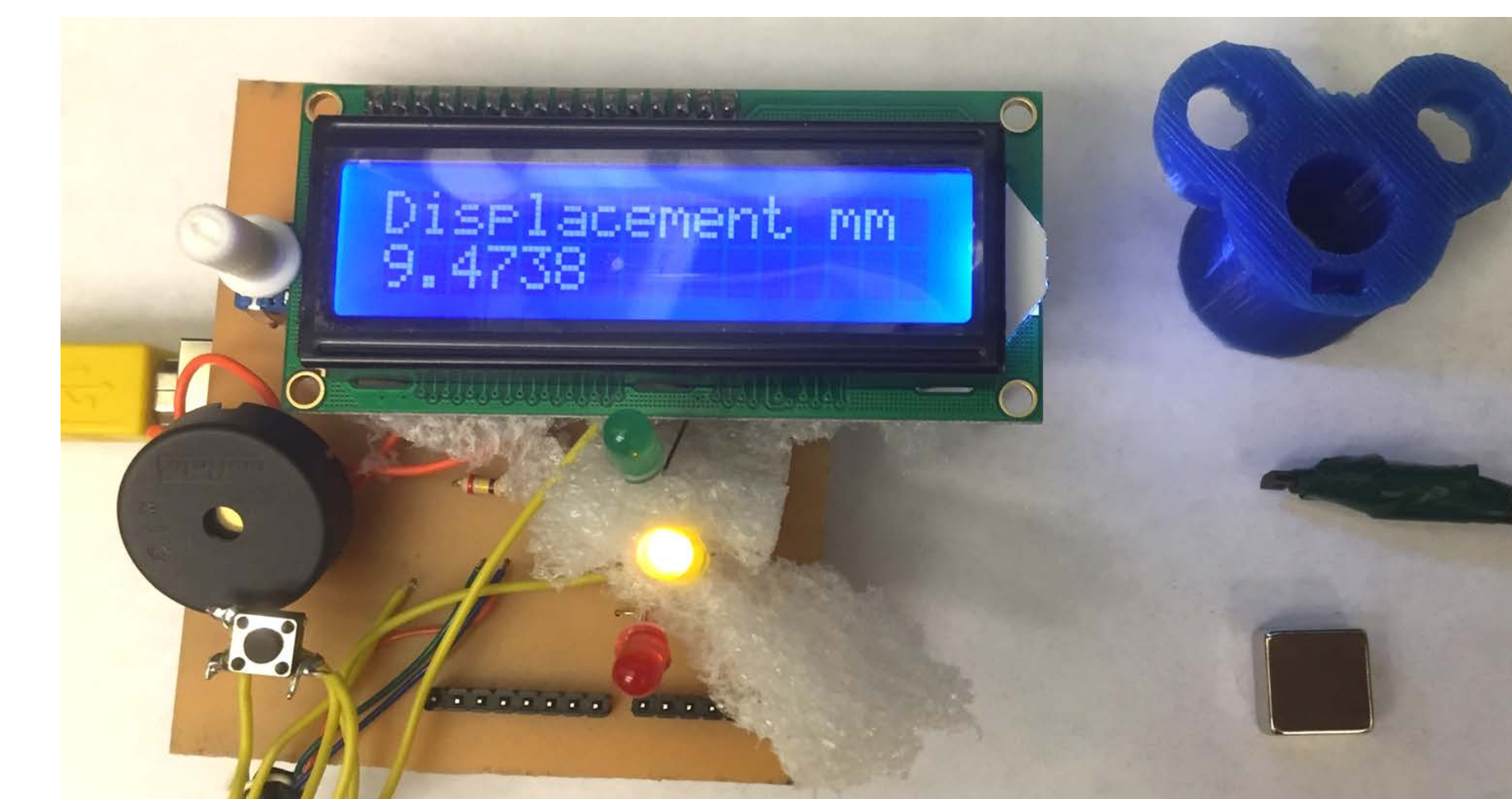
Figure 3: All circuitry, including LEDs and buzzer, were soldered onto an etched board, which shields the Arduino. Testing revealed that the LEDs and buzzer functioned properly, and that the correct displacement values were displayed after programming.
