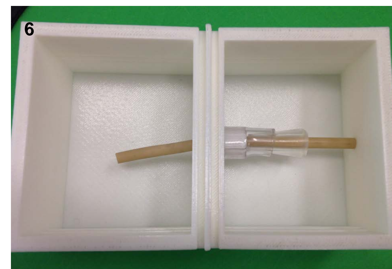
Fig. 6- 3D printed PLA box created for bacterial culture. Left side would receive L. broth and right side would be seeded with bacteria on agar gel.
