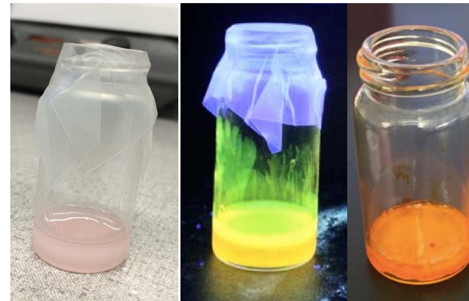
Figure 2: PEGDA hydrogel prior to UV catalysis (Left). PEGDA hydrogel during UV catalysis (Middle). PEGDA hydrogel after 30 minutes of UV catalysis (Right)
