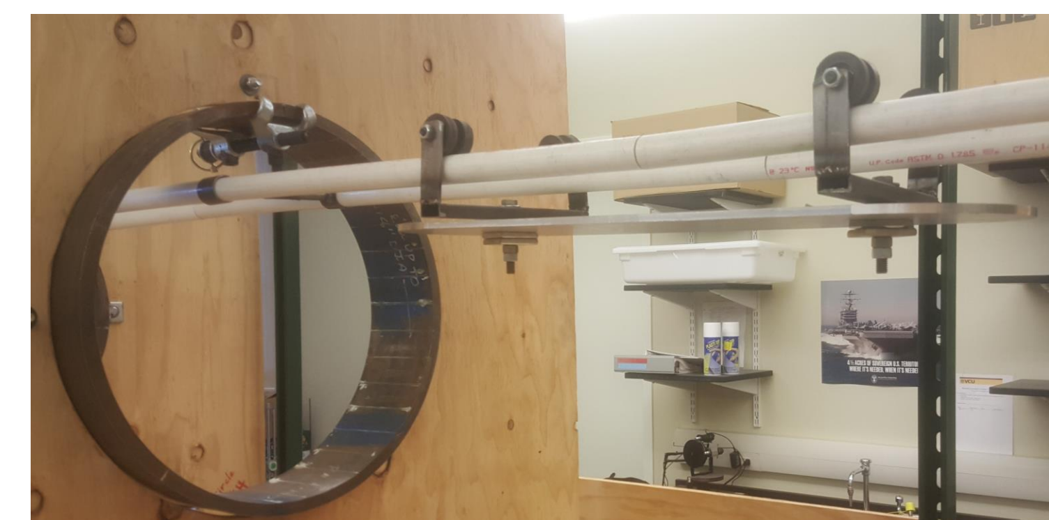
Cart Installed on Rail System
