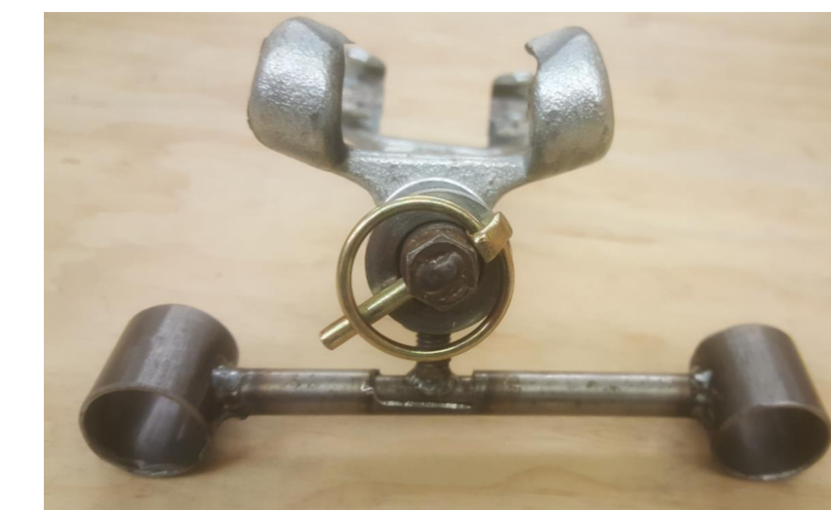
Flange Clamp Assembly Removed
