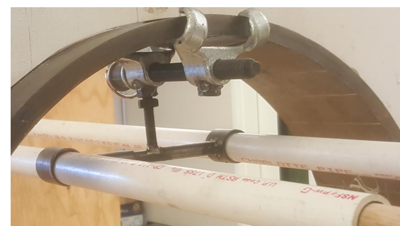
Flange Clamp Installed on Flange
