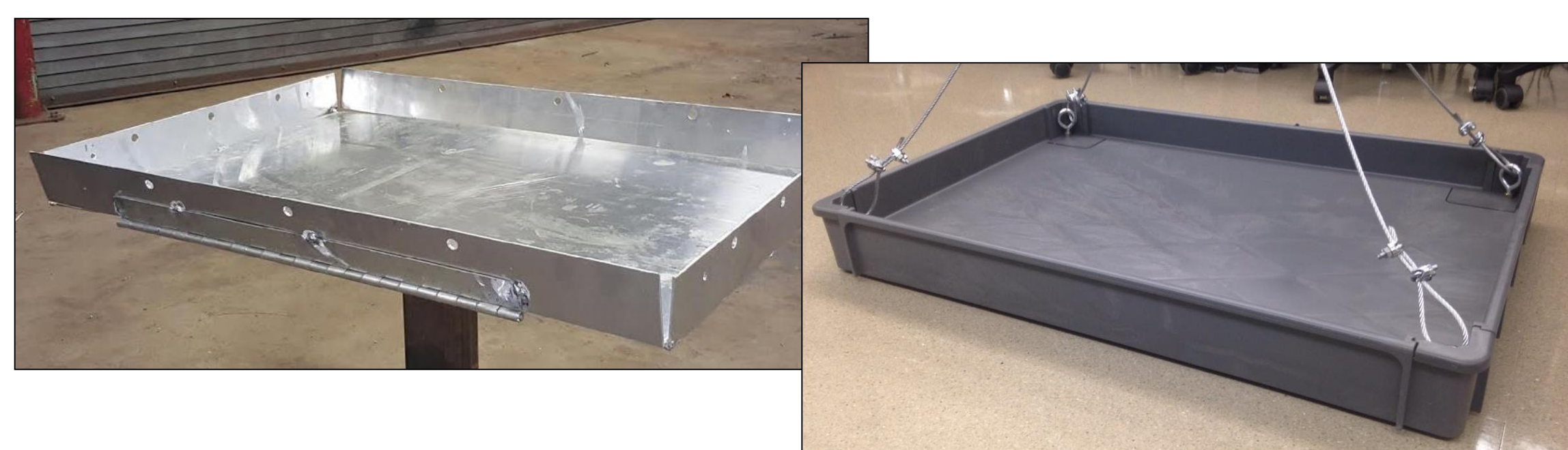
Figure 2: The aluminum cart (left) and the polypropylene cart (right)
