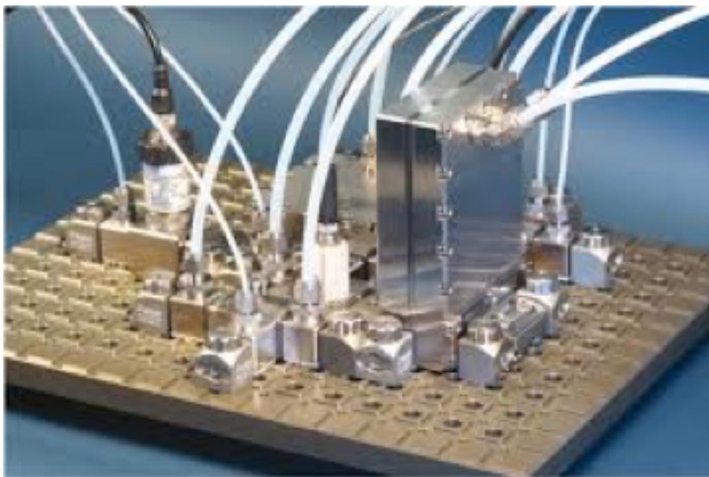
Fig. 2.4.1.1. Modular Microreaction system (MMRS) containing all parts; mixture, sandwich microreactor, inlet/outlet modules, and flanges.
