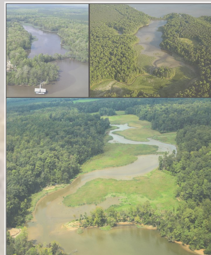
Figure 1. KC Wetland Restoration. Pre-restoration (upper left): Impoundment of KC, former Lake Charles. Transitional (upper right): partial breach in 2007. Restored (lower): partial removal of dam in 2010. By Bukaveckas & Wood, 2014
