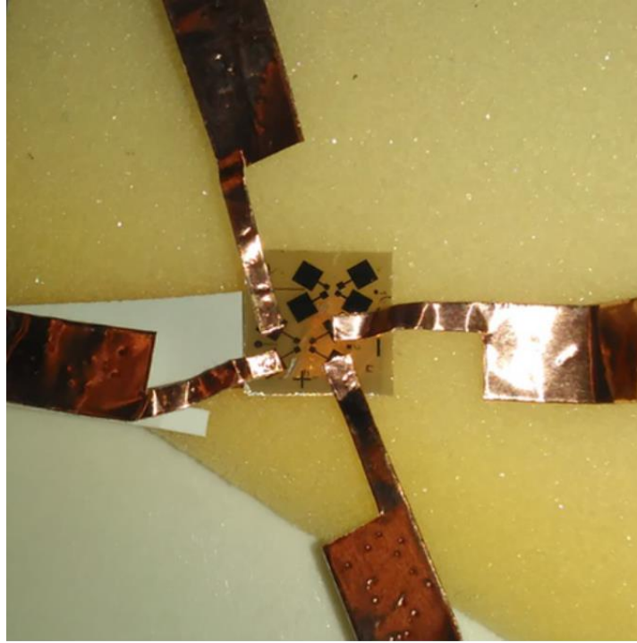
Fig. 4. 2 Experimental setup before application of stress. Copper tape has been used for external contact with the bigger Au electrodes that are deposited on the PMN-PT substrate.
