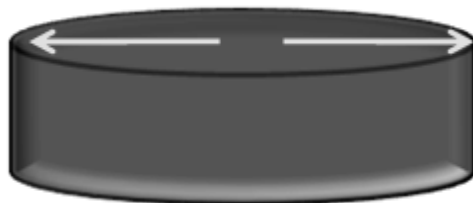
Fig. 1. 1 : The two stable magnetization orientations in a single domain ferromagnet shaped like an elliptical cylinder are shown with arrows.
