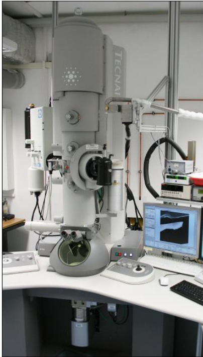
Figure 3.4. The actual image (left) and simplified schematics (b) of the low temperature (S)TEM-CL setup located in University of Magdeburg, Germany which is being utilized in order to study spatial features and defect distributions as well as their optical properties in our project as a collaboration at University of Magdeburg, Germany.
