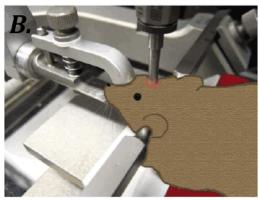
**Figure 2.2. CCI device.** Photographs representing the (A) Controlled Cortical Impact injury device and (B) position of the animal during injury.
